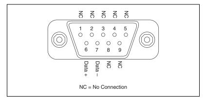
Figure 2-6. FBUS-HSE/H1 LD Connector Pinout
